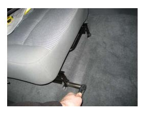
Remove front bolts on passengerside seat and position base assembly in front of seat mount brackets.
